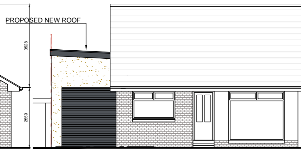
PROPOSED SOUTH ELEVATION SCALE 1:100
