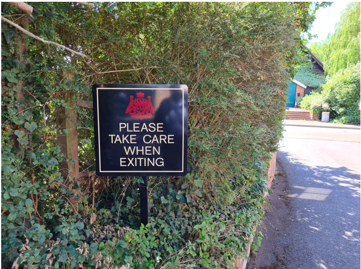
Photo P – Post sign close to driveway exit. Sign H610mm, W610mm. Post and sign H1200mm.
