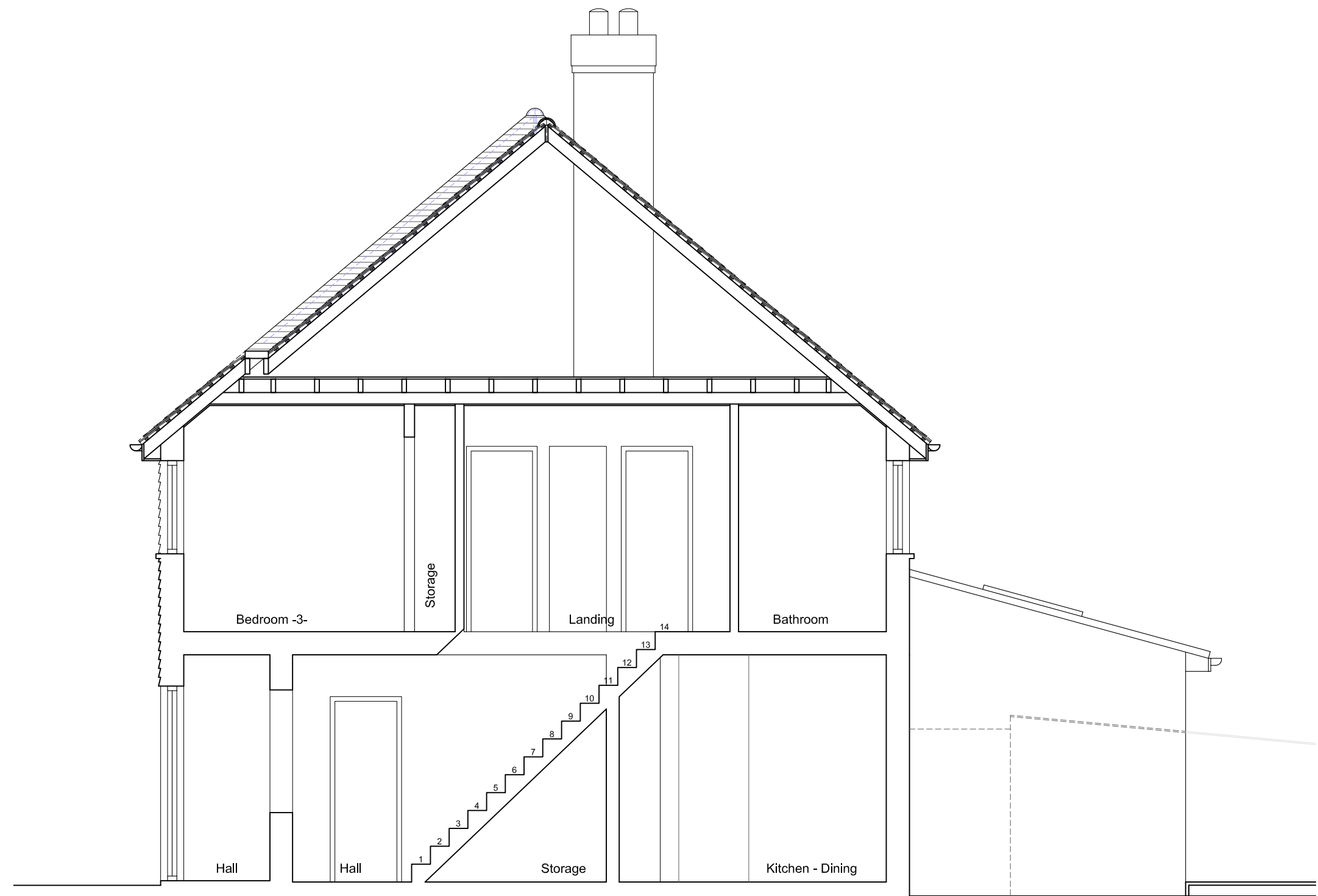
EXISTING SECTION A-A
