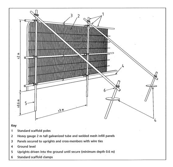
Where practicable, the uprights should driven securely into the ground to a minimum depth of 600mm. However, where site conditions prevent this an above ground stabilizing system can be adopted. Examples are given in Fig below.
