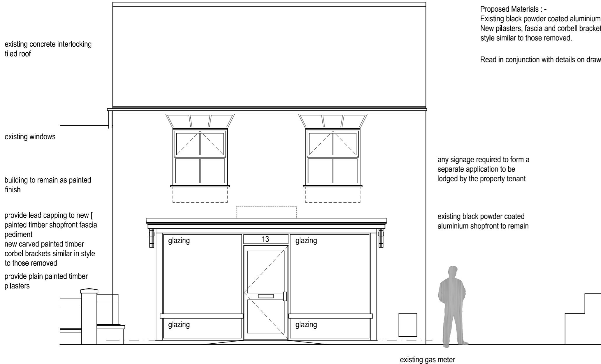
Elevation to High Street as Proposed 1:50
