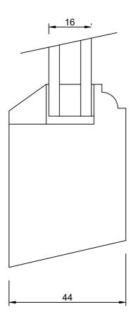
Selden, Ground Floor Flat, The Old Vicarage. Gibraltar Hill, Lincoln Windows D, E & F Drawing showing cross section of sash section, bottom rail section and double glazed units with beaded glazing. Scale 1:1
