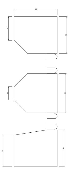
Selden, Ground Floor Flat, The Old Vicarage. Gibraltar Hill, Lincoln Windows A,B & C Drawing showing cross section of typical frame, mullion, transom and cill sections.
