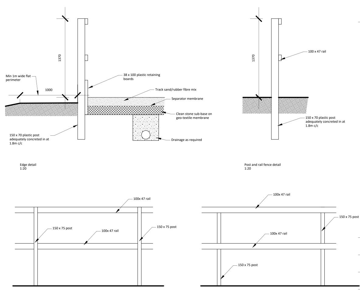
Post and rail fence external elevation 1:20
