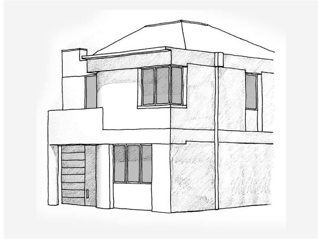
Sketchbook: Proposed sketch view showing frontage design. Front bay, corner window, setback entrance and canopy used to create visual depth and relief that reinforces the character of the area. The eaves line acknowledges those of its neighbours. Rainwater pipes and steps in the render reinforce the depth of the front bay, providing further visual quality and character.
