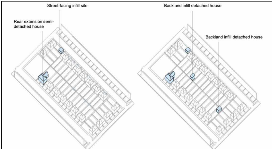
Figure 3—GLA Small Sites Design Code —Figure 2.4 Opportunities for incremental housing development within semi-detached contexts
