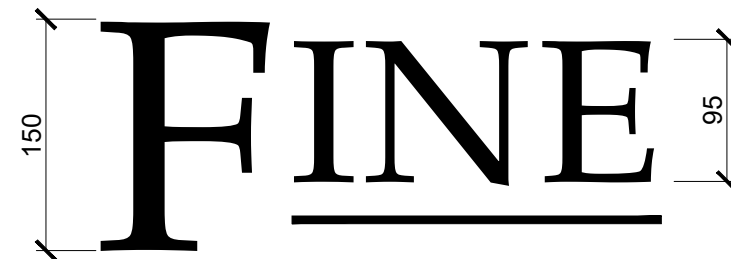
③ FASCIA SIGN LETTERING - AS PROPOSED Scale: 1:5
