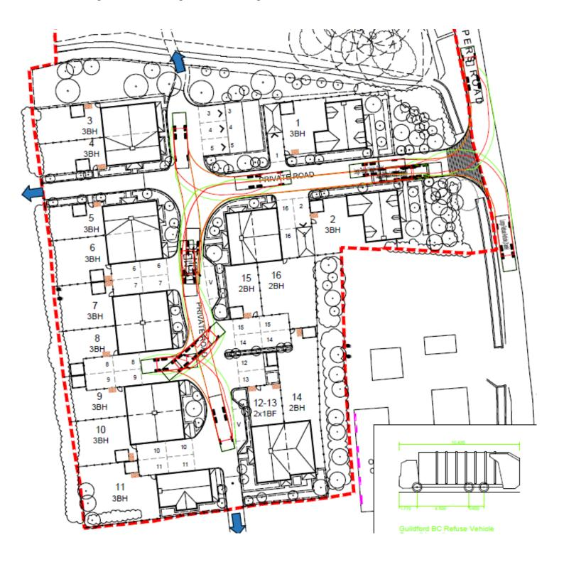
In this southern part of the site, reference to the extract from the proposed site plan (PL-01 Rev M) below indicates that plots 1-16 inclusive can be served directly by the manoeuvring refuse collection vehicle (rcv) as it follows the above tracking route.
