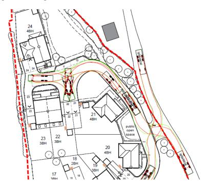
Refuse vehicle moving to southern part of northern half of site manoeuvring in turning head and exiting in forward gear
