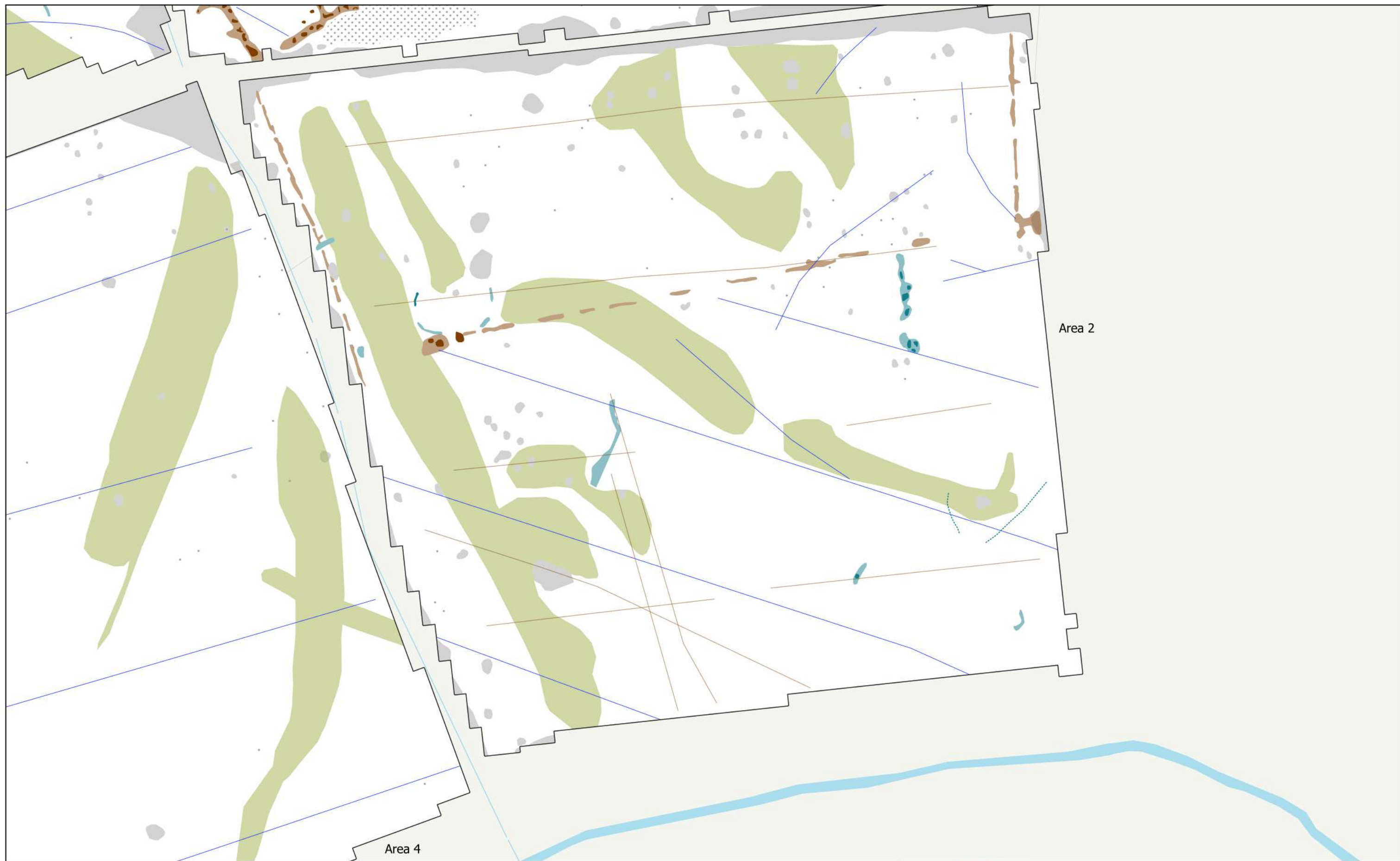
MSTQ1118 - Burstead Solar Farm and Battery Storage Figure 33 - Magnetic Interpretation (Areas 2 & 4) 1:1,500 @ A3 Copyright Magnitude Surveys Ltd 2022 Contains Ordnance Survey data © Crown Copyright and database right 2022
