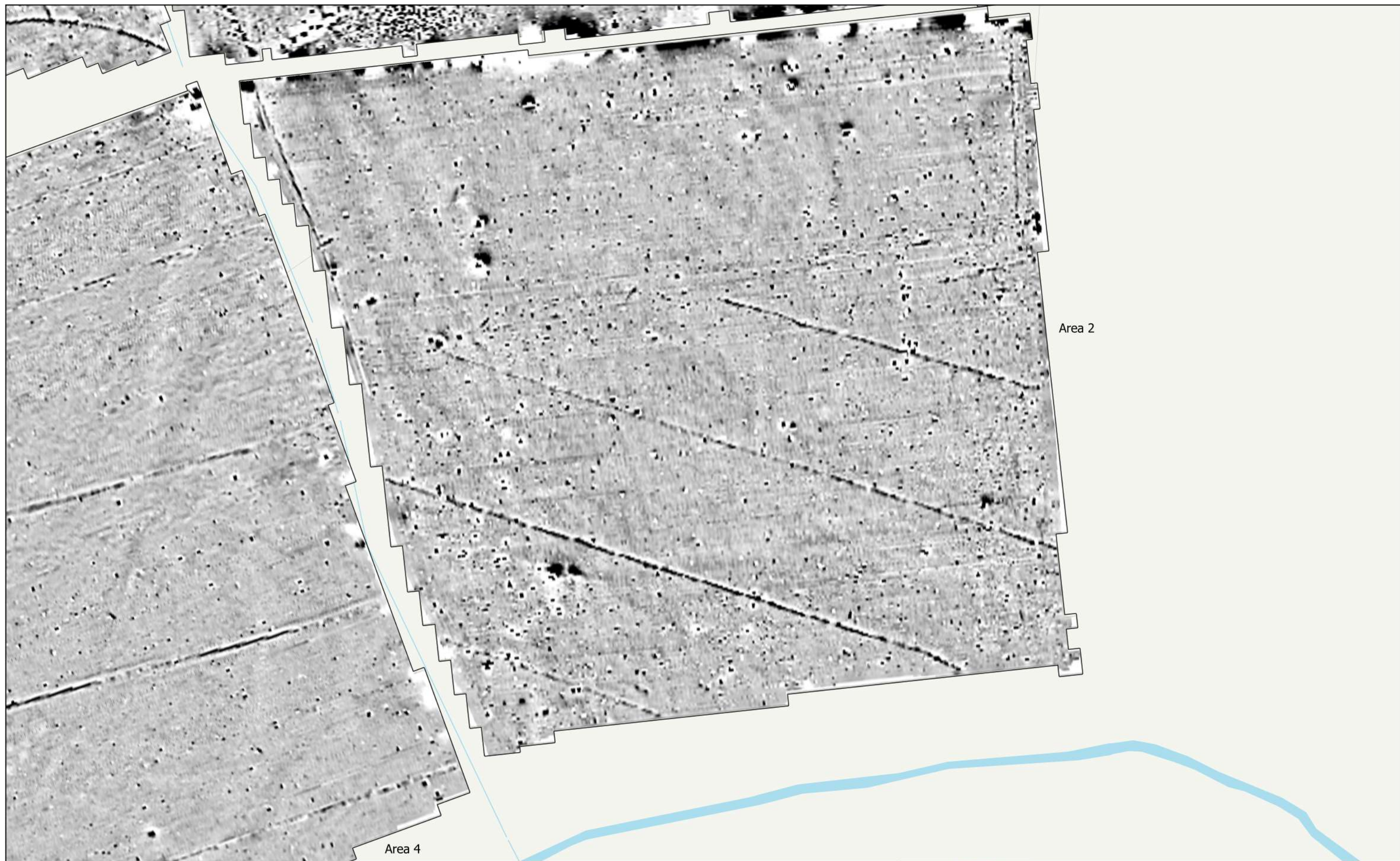
MSTQ1118 - Burstead Solar Farm and Battery Storage Figure 32 - Magnetic Gradient (Areas 2 & 4) 1:1,500 @ A3 Copyright Magnitude Surveys Ltd 2022 Contains Ordnance Survey data © Crown Copyright and database right 2022
