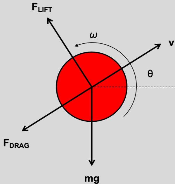
The aerodynamic forces of drag ( $F_D$ ) and lift ( $F_L$ ) are proportional to the ball’s velocity relative to the air flow, frontal area, air density and the drag coefficient respectively lift coefficient. The forces are defined as:
