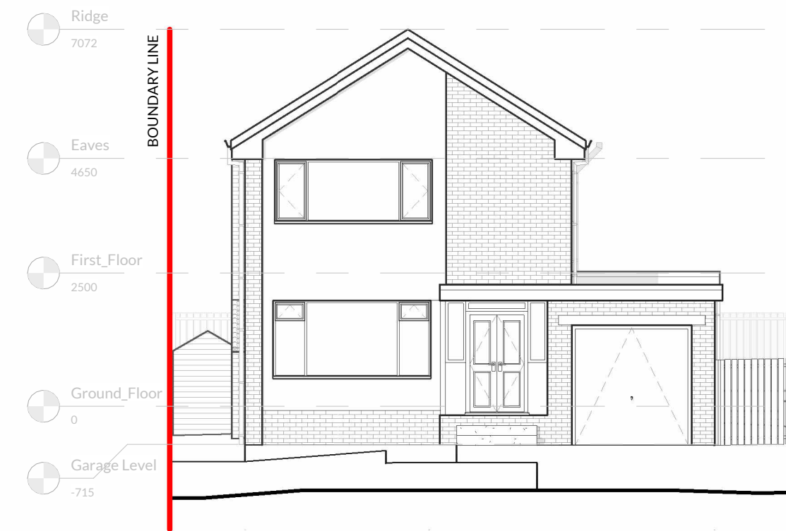
01 - South Elevation (Front) 1:100
