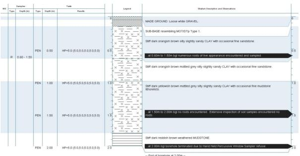
End of borehole at 2.00m -Borehole completed by hand held percussive window sampler: Roots encountered to 1.50m bgl. Groundwater strikes not encountered, PEN = Hand Penetrometer (kg/sq.cm).
