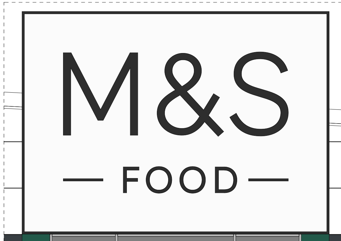
3D HALO ILLUMINATED BLACK LETTERS (RAL 9005) ON A WHITE (RAL 9003) FLEX FACE SIGN.
