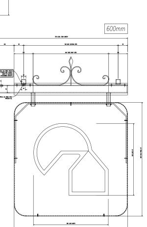
25mm X 3mm MILD STEEL SCROLLWORK WELDED TO PROJECTING ARM FINISHED XXXXX
