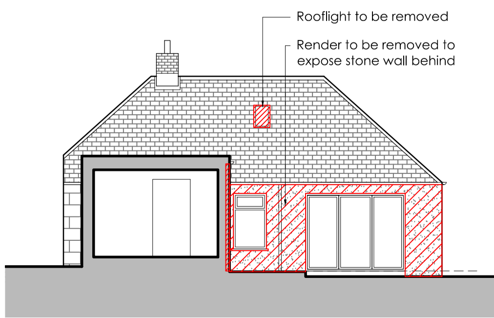
Demolition West Elevation from Courtyard at 1:100
