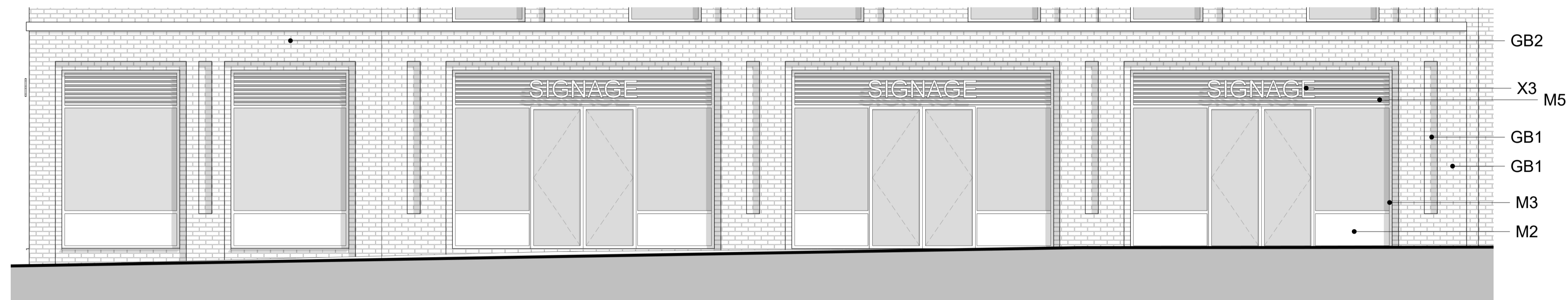
2 Block A_GA Elevation_High Street_1-50_Retail Shopfront 1 : 50
