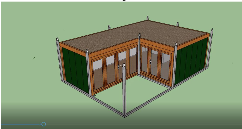
Vertical sections fitted at key points around structure with lifting points visible.
