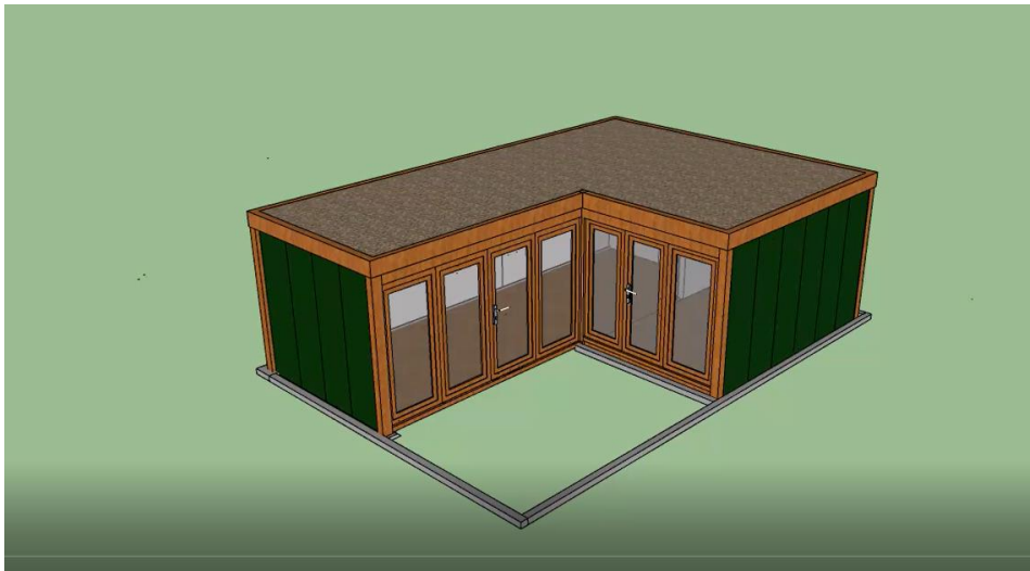
Steel cradle sections formed around edges and beneath structure.
