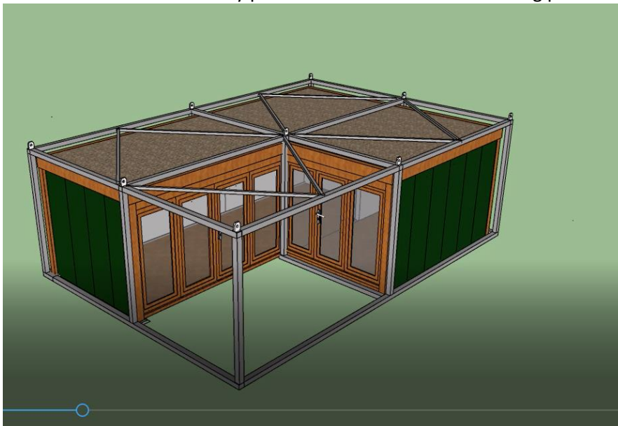
Vertical sections connected above roof by steel cross-sections to retain cradle rigidity.
