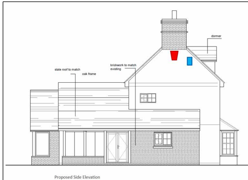
Figure 11. Proposed roost features on extended Farmhouse (green rectangle = lifted ridge tile; blue rectangle = gap recreated into soffit at same location as existing Common Pipistrelle day roost)
