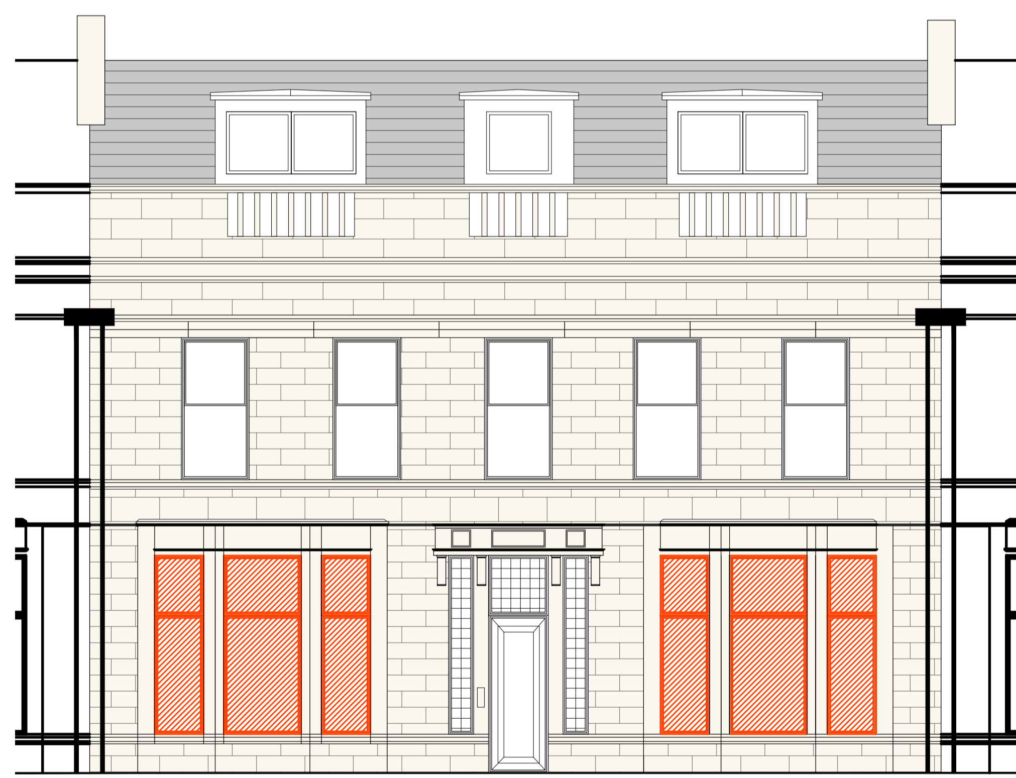
Front Elevation as existing - Downtakings Scale 1:50
