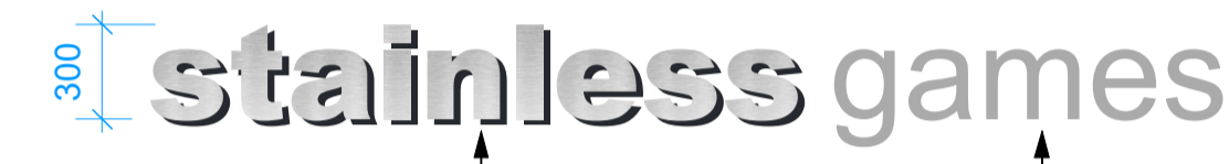
13 Surface mounted stainless steel signage Hand painted grey signage
