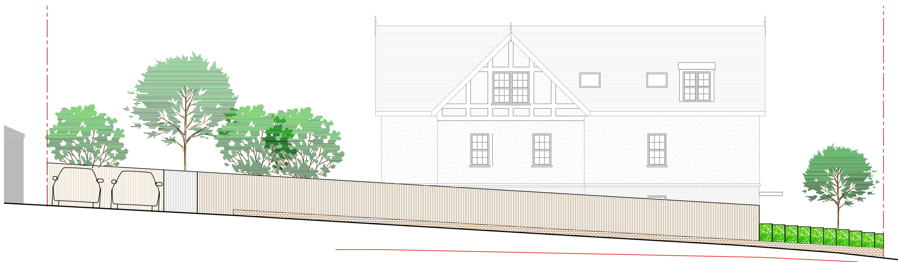
Proposed Side Elevation Showing Boundary Treatment Scale 1:100
