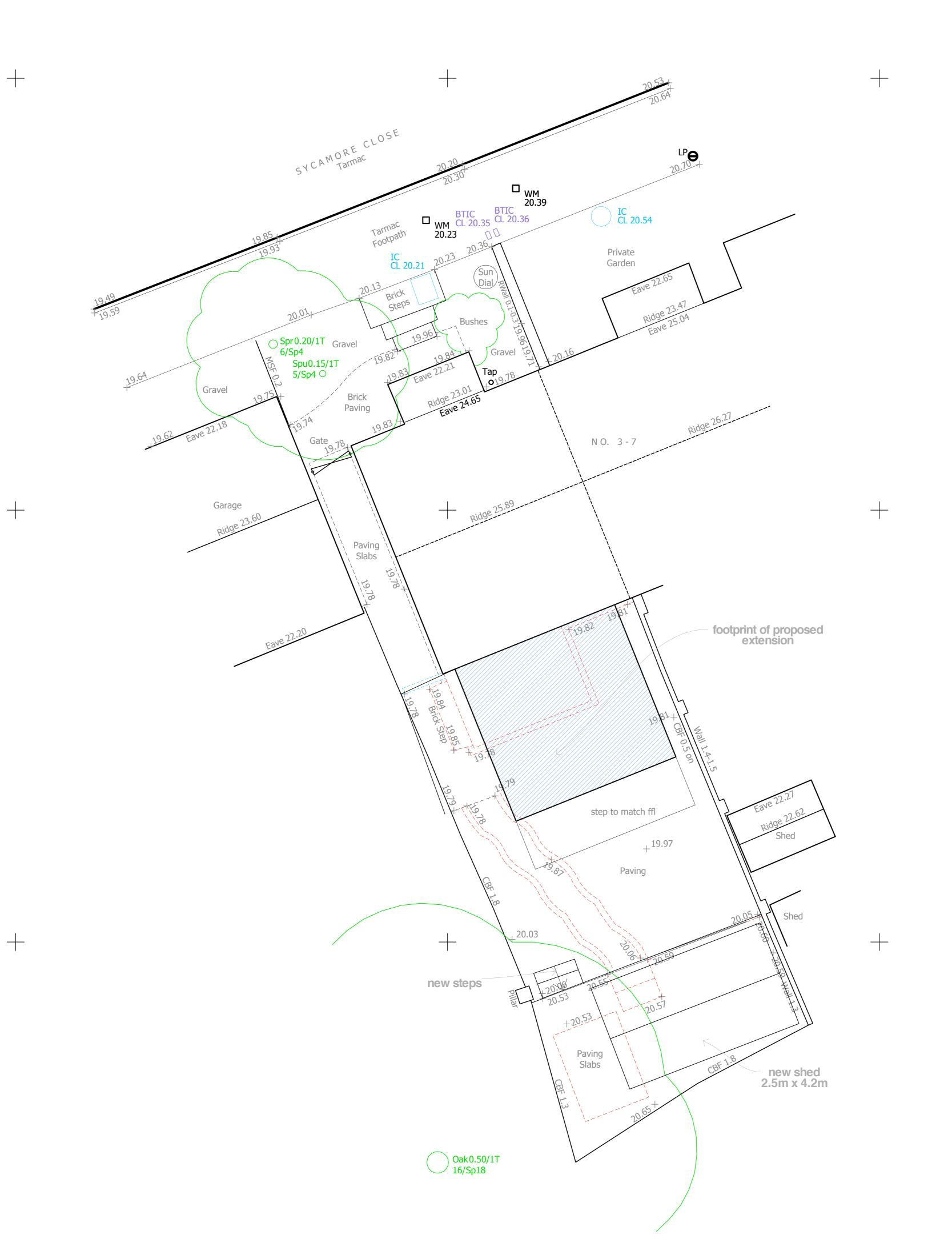
Proposed Site Plan scale: 1:50 @ A1
