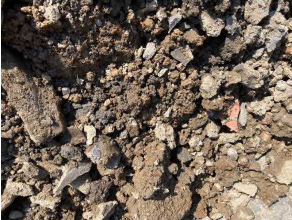
Photograph 99 Description: Spoil encountered in trial pit TP36 Date: 08/06/2023 Location: Lower quarry bench
