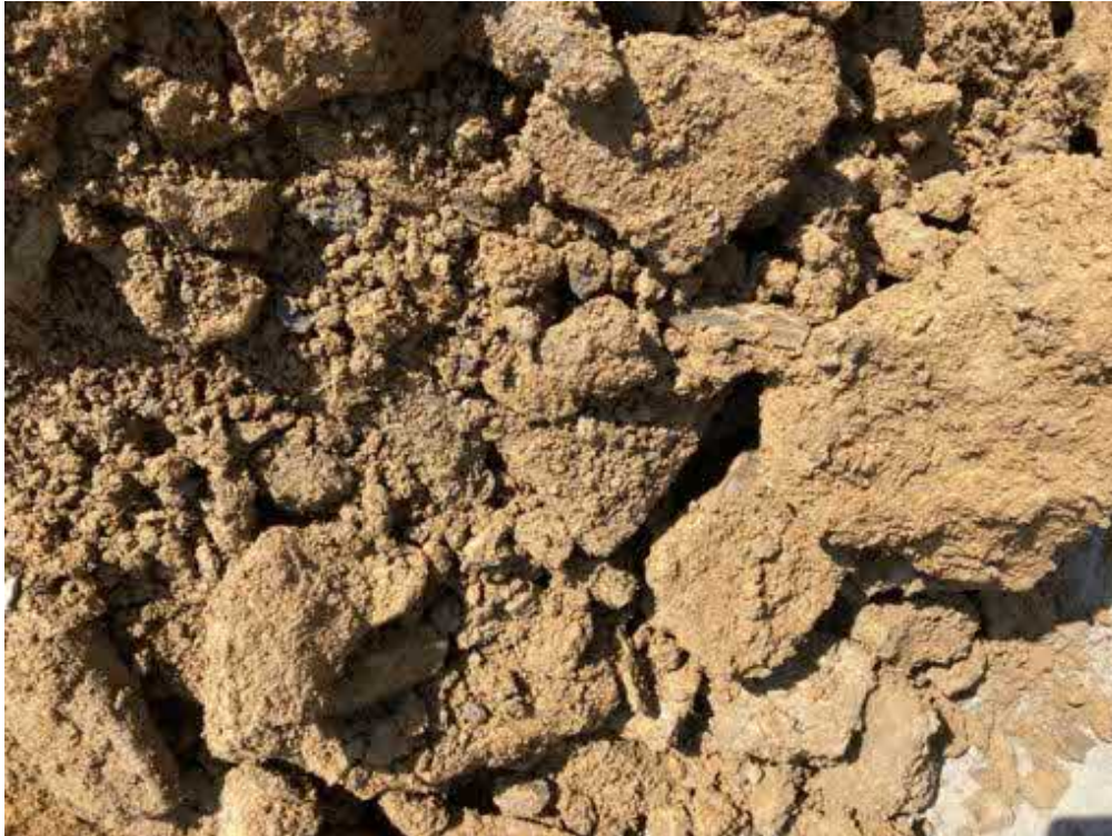
Photograph 107 Description: Sandy clayey silt encountered at the base of trial pit TP40 Date: 08/06/2023 Location: Lower quarry bench
