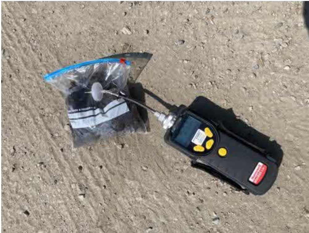
Photograph 111 Description: Example of PID headspace testing Date: 08/06/2023
