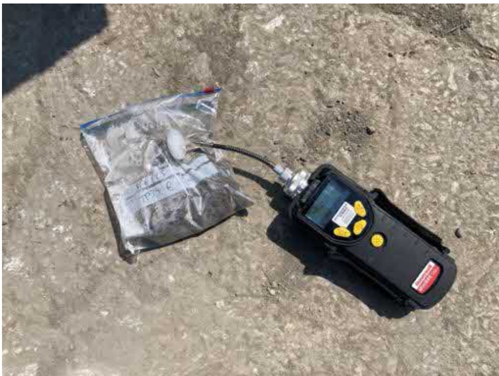
Photograph 110 Description: Example of PID headspace testing Date: 08/06/2023
