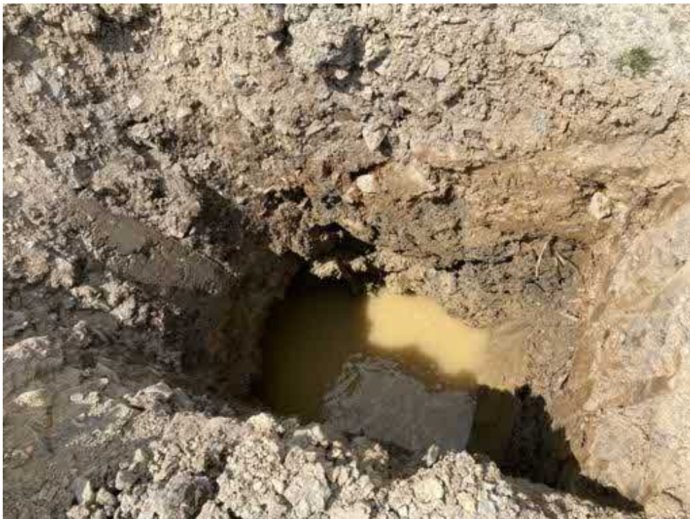
Photograph 18 Description: Trial pit TP03 (including perched water) Date: 07/06/2023 Location: Upper quarry bench
