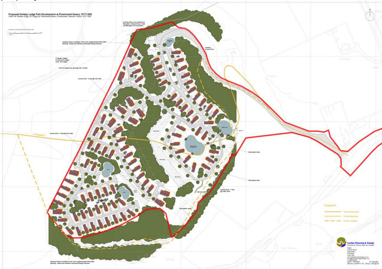
Figure 36. Layout plan, illustrating the Lodges in muted environmental colours in a low density informal layout in a heavily landscaped setting with expanded buffer planting around the periphery and within the site.
