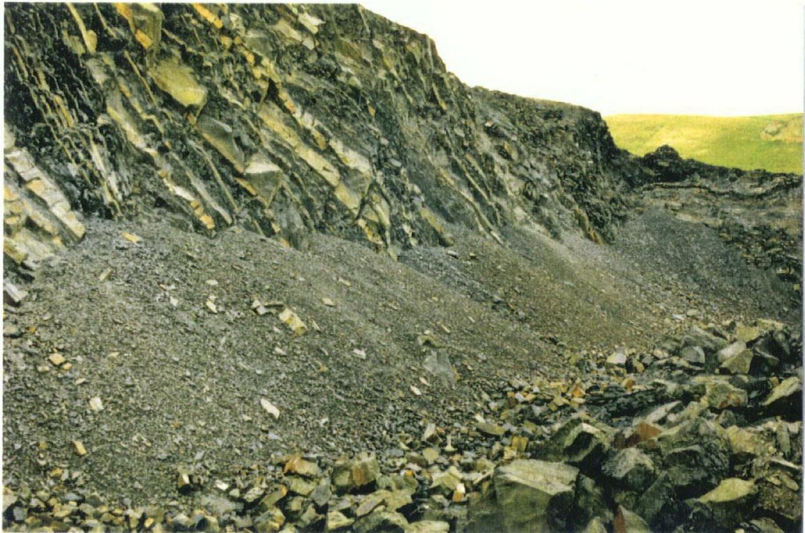
Figure 29 Accumulation of scree at base of unstable faces along the upper level. The continued build-up of this material will eventually result in the loss of exposure. Without further quarrying at the site, some clearance may eventually become necessary.
