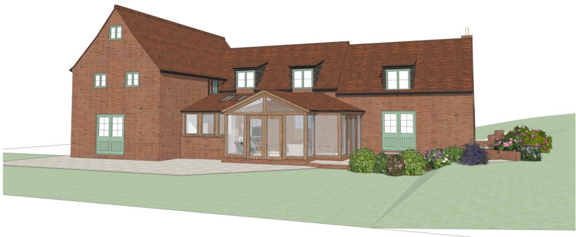
3D view of the proposed extension with tiled roof and projecting bay to frame views over Aylesbury Vale
