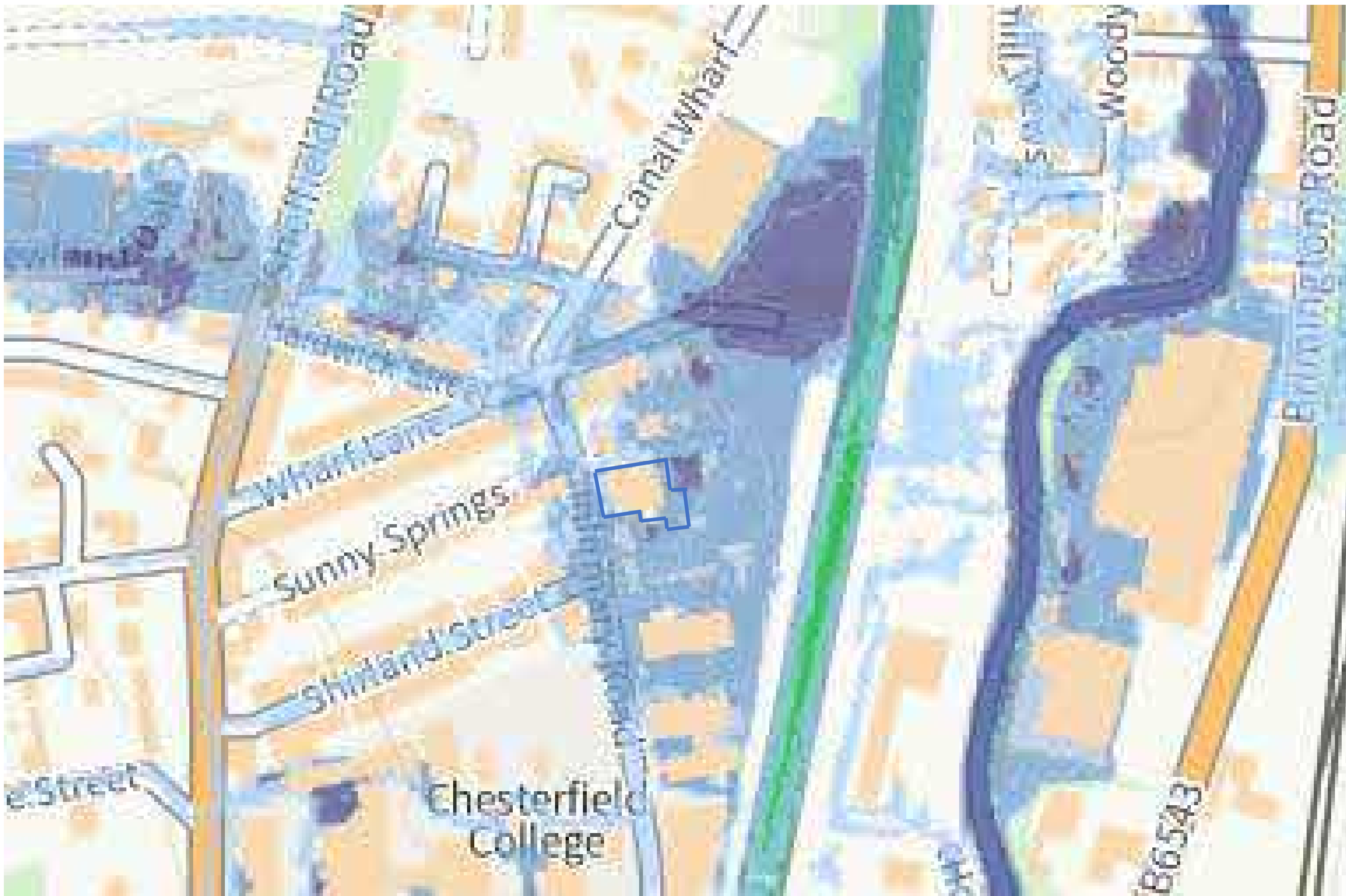
Surface Water Flood Risk Map – Low Risk Scenario (1 in 100 to 1 in 1000 Years- Equivalent to Flood Zone 2)
