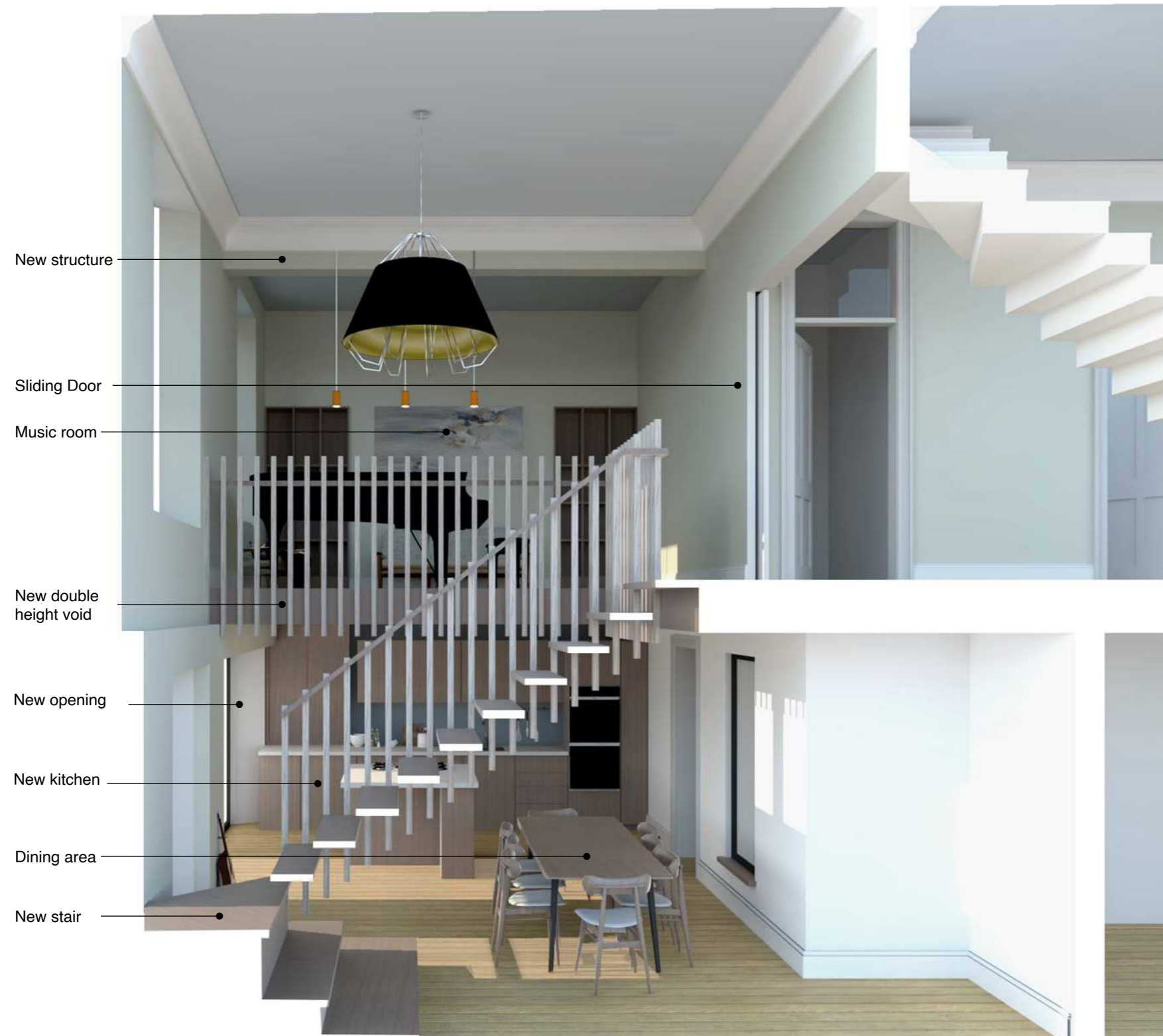
* 9 Circus Place | Section cut through new stair / music room / diner / kitchen | proposed family space
