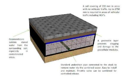
Figure 7: Block Permeable Paving with Geocellular Module
