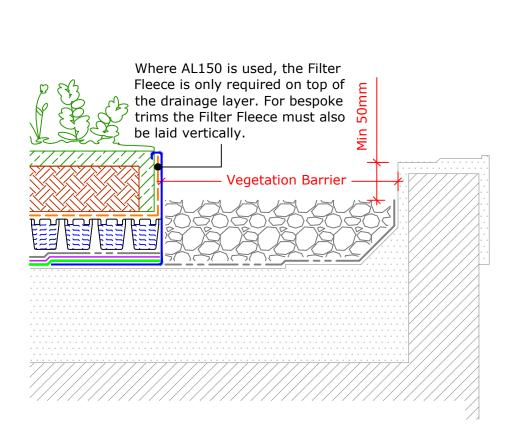
Perimeter Kerb (Drg.No: D0901/03-00W\_0-4Deg\_002-ExtInt-S-DB\_001)
