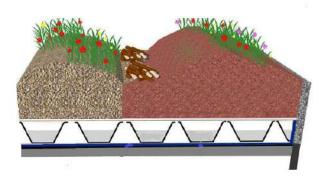
Figure 4: Biodiverse green roof diagram (University of East London)
