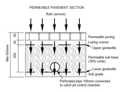
Figure 6 Block Permeable Paving with sub-base
