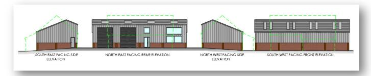
The proposed will be a steel framed building and will be built with natural grey box profile tin sheets to the upper walls to match the existing main building on site with a rural blend red brick the lower walls. The roof will be corrugated sheets light grey in colour with GRP roof lights. 2 metal roller shutter doors in grey and the UPVC doors and windows will be double glazed.
