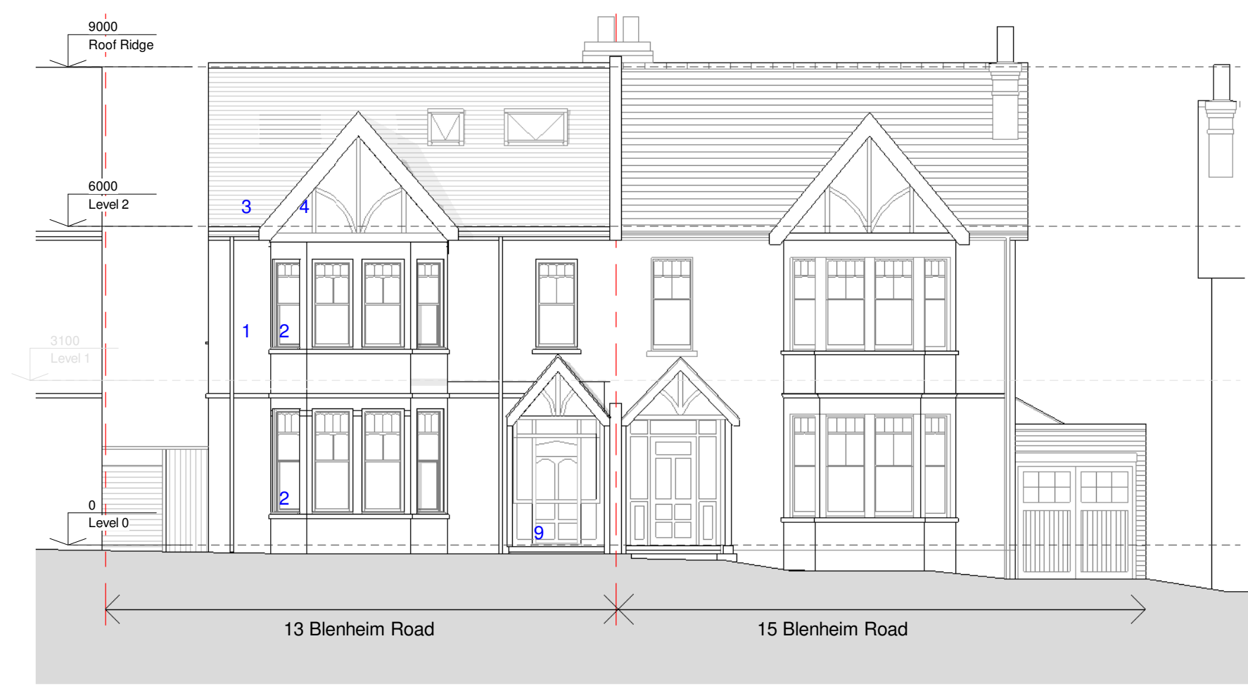
Existing Front Elevation 1 : 100
