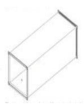
The Ductwork is manufactured from galvanised mild steel sheet, folded and lock formed with flanged construction in accordance with D.W.144 specification or can be spiral round ductwork.
