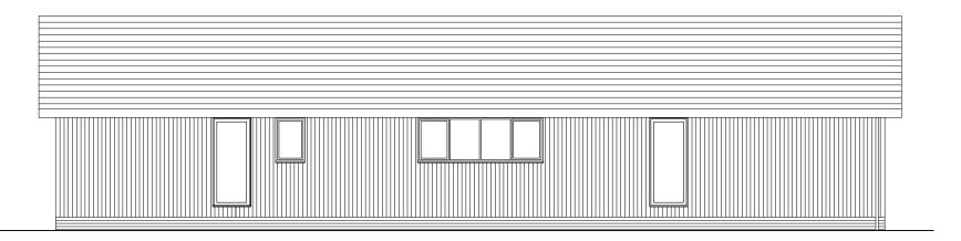
The Lodge will be clad with vertical larch cladding, with anthracite grey PVC double glazed windows. The roof will be a snap-lock, standing seam steel roof (Catnic Urban) also in anthracite.
