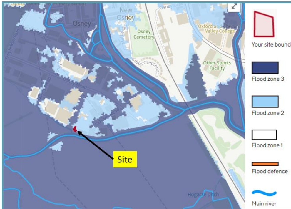
Figure 8 EA Flood Risk Map for Planning, showing site located in Flood Zones 2 and 3.
