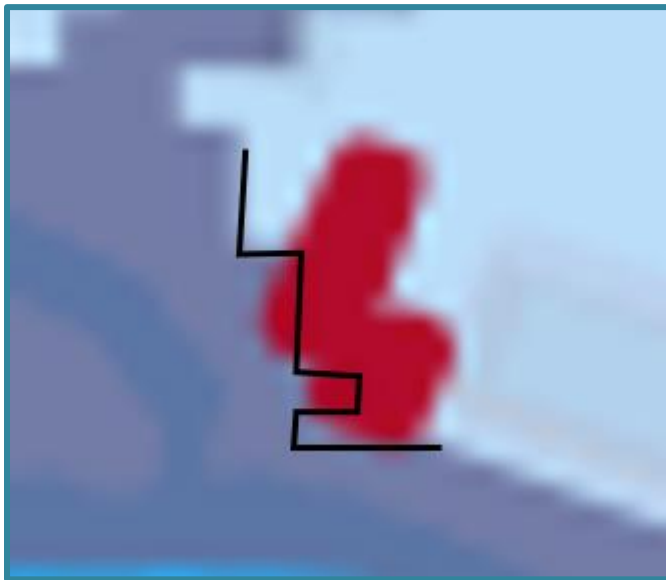
Figure 9 Expanded EA Flood Map for Planning; the blurred outline is from the EA Flood Map. The black alignment is the division between Flood Zones 2 and 3, as traced.
