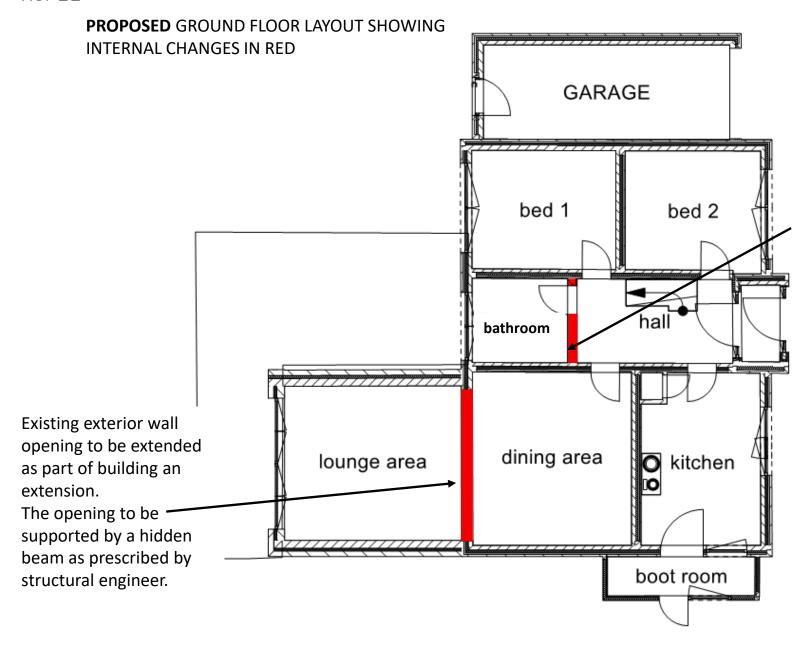
New bathroom wall to replace the existing wall to increase the size of the bathroom to allow the installation of a walk in shower.
