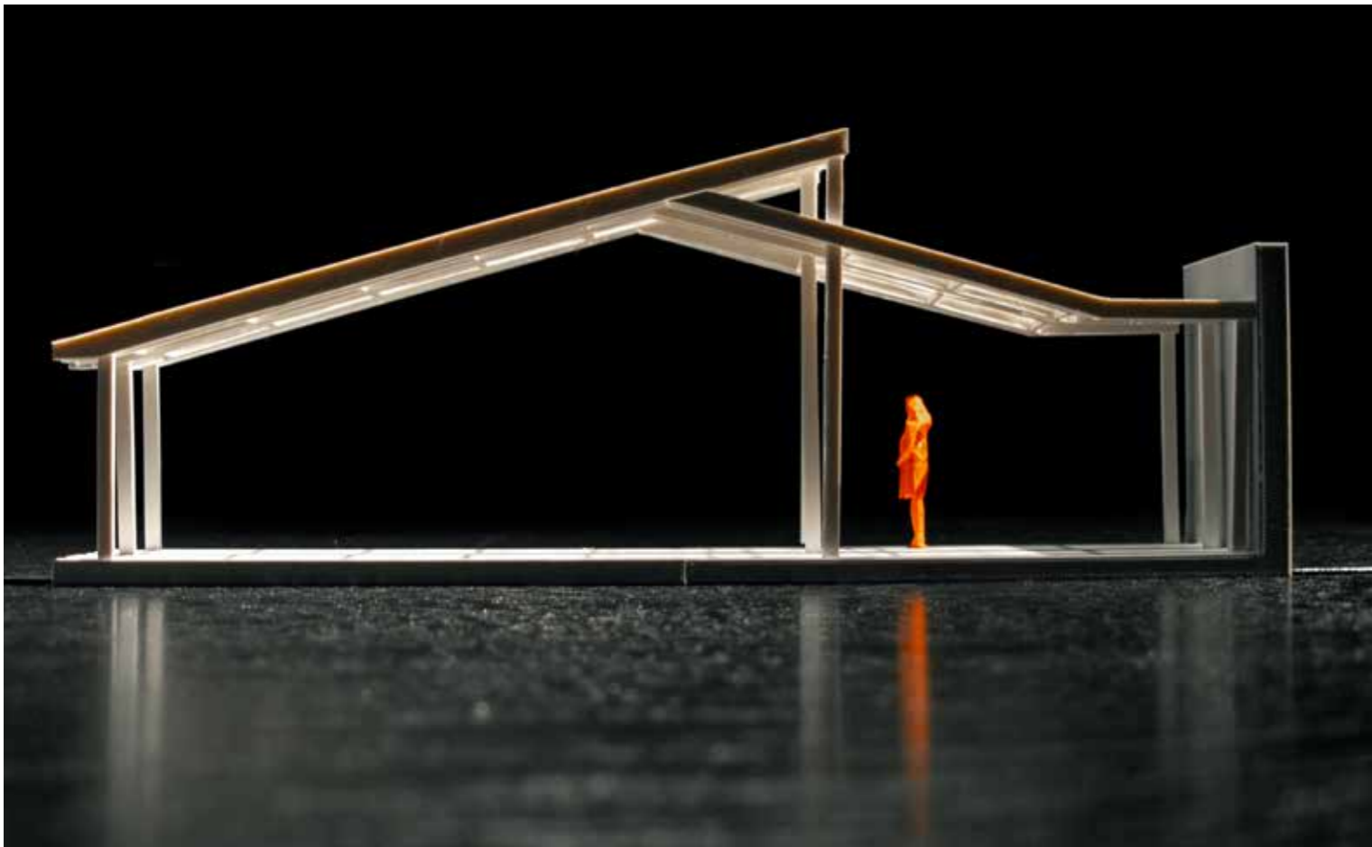
A series of truss options has been explored to establish an arrangement which balances visual interest (internally), a large clerestory and minimal visual impact from the street.
