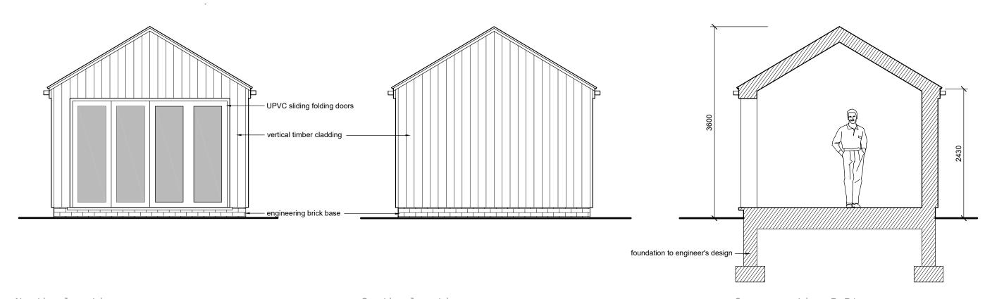
North elevation South elevation Cross section D-D'
