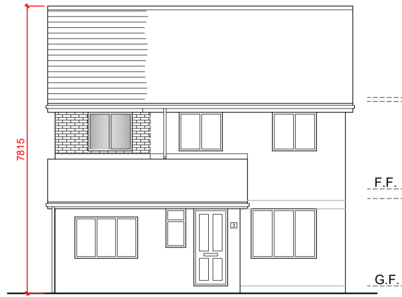
Proposed Front Elevation Scale: 1/100
