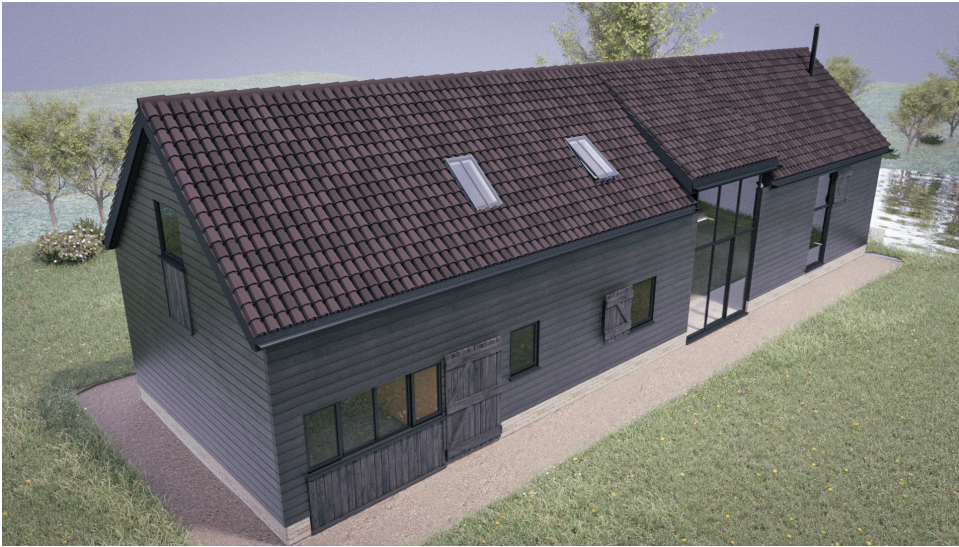
Fig.8 3D render of Velux Heritage conservation roof windows in The Barn. (Please note: due to software limitations, the tiles shown in these 3D renders are not an exact representation of the actual tiles to be used/retained).
