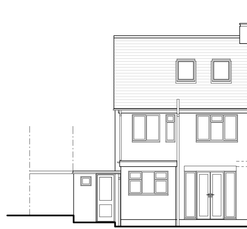
REAR ELEVATION AS EXISTING Scale 1:100
