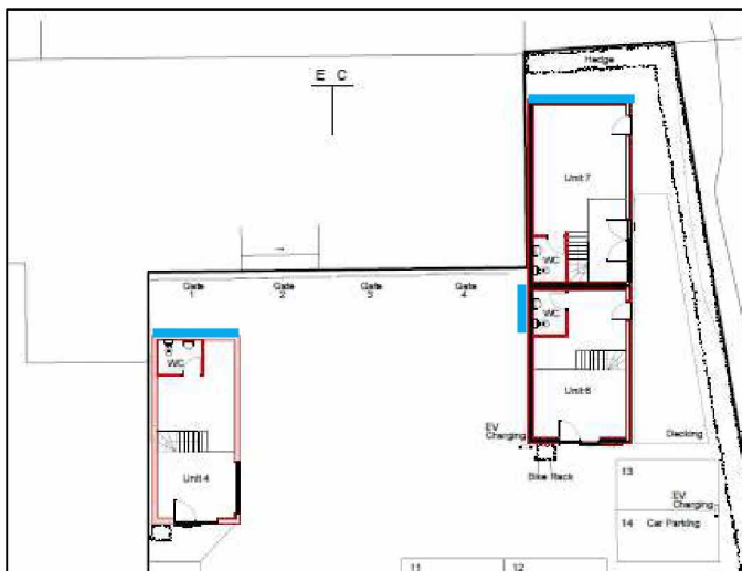
Fig.6: Recommended location for external mechanical plant for units 4, 5 & 6 (labelled 6 & 7) indicated by a blue line.
