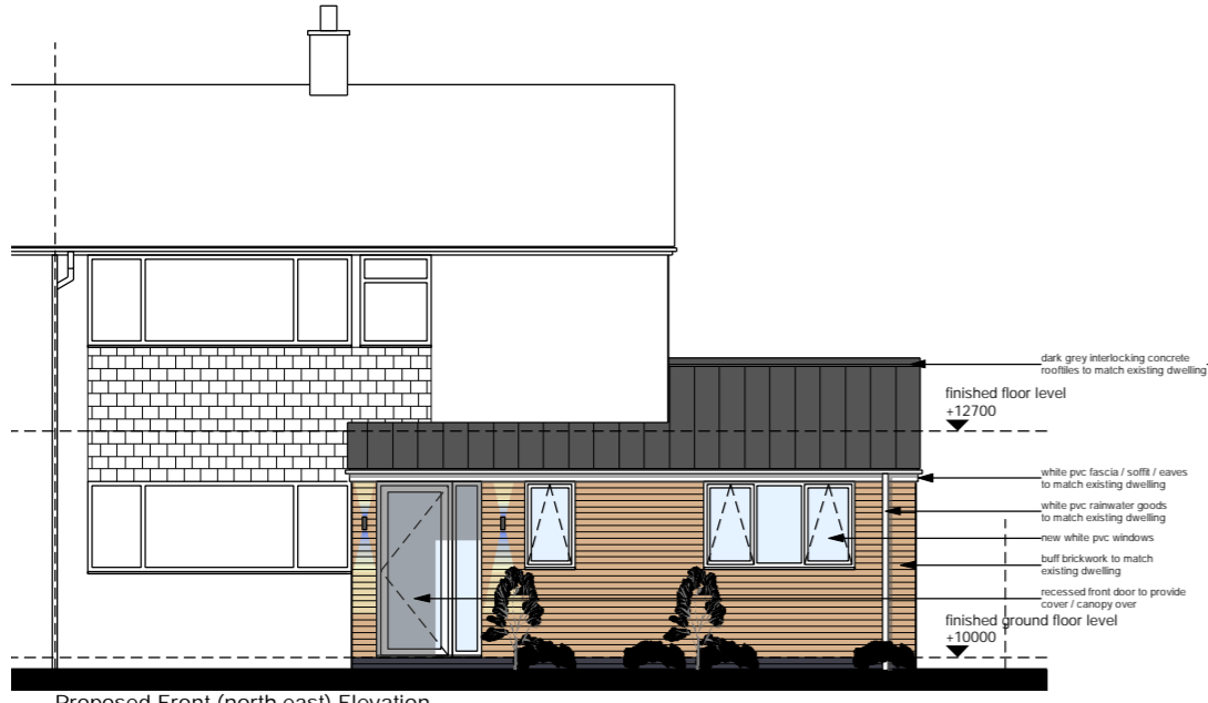
Proposed Front (north east) Elevation (scale 1:100)
