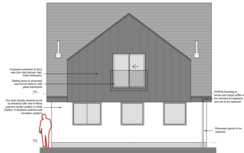
Proposed North Elevation 1:100 @ A3
