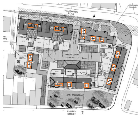
Figure 3 – Proposed Roof Plan showing Location of Proposed PV Panels
