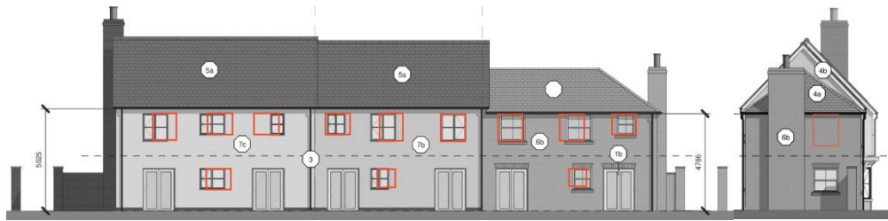
affected windows of Plots 1-3 showing approximate permitted window outlines in orange (rear and west elevations)
