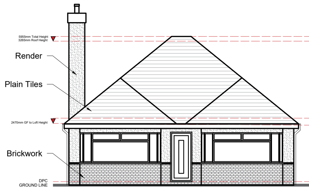
Existing South-West Elevation Scale: 1:100
