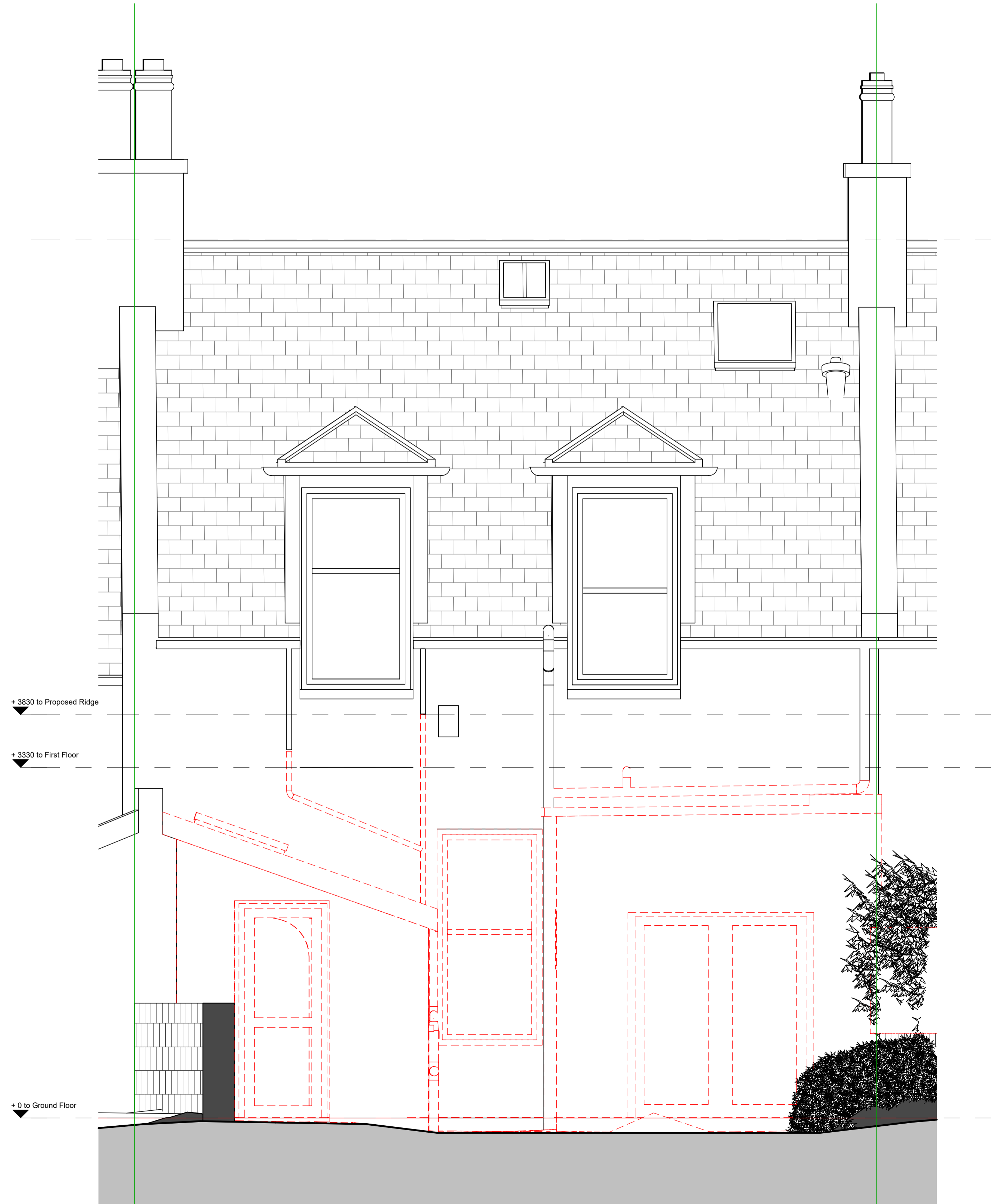
East Elevation Demolitions
